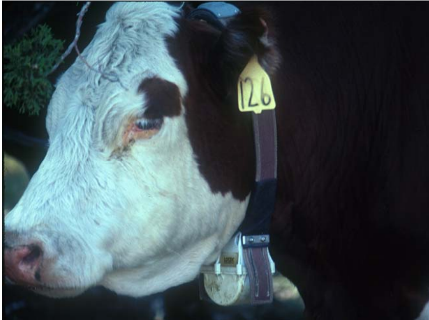
Figure 1. Beef cow no. 126 wearing a GPS collar used to determine her precise location and activity at programmed intervals on the Northern Great Basin Experimental Range.
