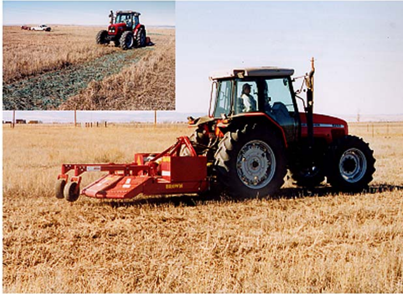
Figure 1. The Brown Brush Monitor™ mows and applies herbicide in a single pass.
